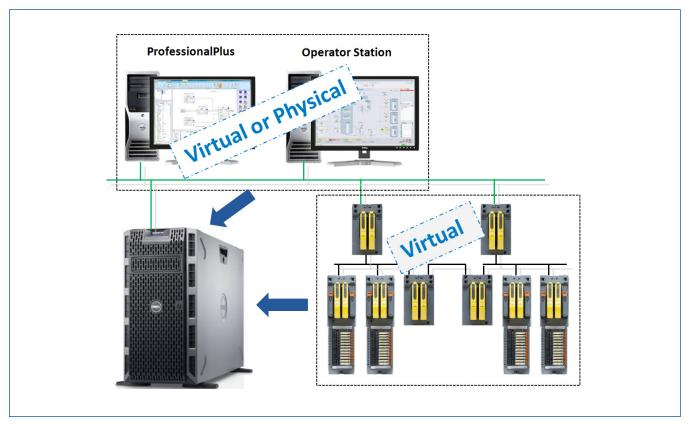
The DeltaV SIS system provides the ability to virtualize hardware components for DeltaV SIS with Electronic Marshalling to facilitate the development and testing of safety logic.
